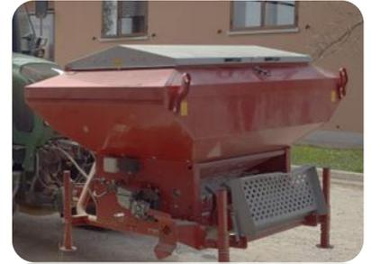
Integration carried out by **Sfoggia (Italy)**. It allows to control the distribution of granular fertilizer, thanks to the use of the **PCS W1** system.
