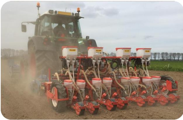
Another application from the company **Kramer (Netherlands)**. It allows to control the whole planting and fertilization process directly from the terminal of the **PCS 200** system. The control of the **individual planting distance** for each planter row allows to maximize the production.
