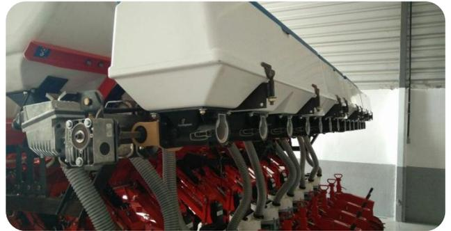
This system, developed thanks to the partnership with the company **Fertisystem (Brazil)**, allows to distribute a special sulfur-based fertilizer in an **extremely accurate** way.
